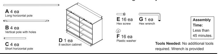
**STEP 1.** Assemble the left frame section by attaching two short horizontal poles (C) to two vertical poles with holes (B). Use plastic washers (F) between the poles and attach using hex screws (E). Use the holes that are closer to the center of (B). Repeat this process for the right frame section.
