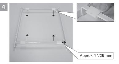
Mount 4 clips on the top frame, with the holes towards the inside. Make sure that the clips are approx. 1''/25 mm from each side. (See arrow above.)
