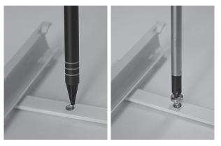
Remove the drawer, mark hole placement and mount the galvanized screws into the cabinet.
